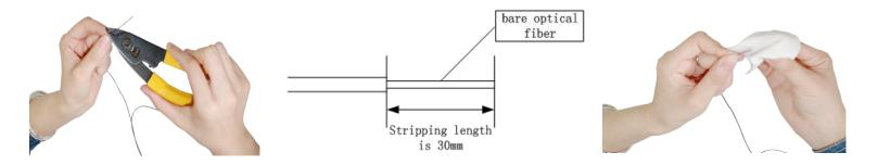
Use the smallest hole of 3-hole stripper to stripe down the coating layer of fiber(Preserve 3-5mm of coating layer), the length shall be about 30mm.
