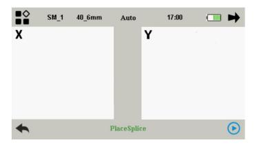
Optical fiber observation interface: Push the power switch then the indicator on the operation panel will turn to red and the buzzer will be sounds like "Di Di". All motors will return back to their initial positions and the fiber observation interface shows.
