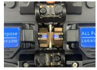
③Put fibers and close the cover the self-test will be on. Normally the test will continue for 2 minutes. Please observe the notice on screen, if the test fails please operate according to instructions on screen and retry it(Step ①).
